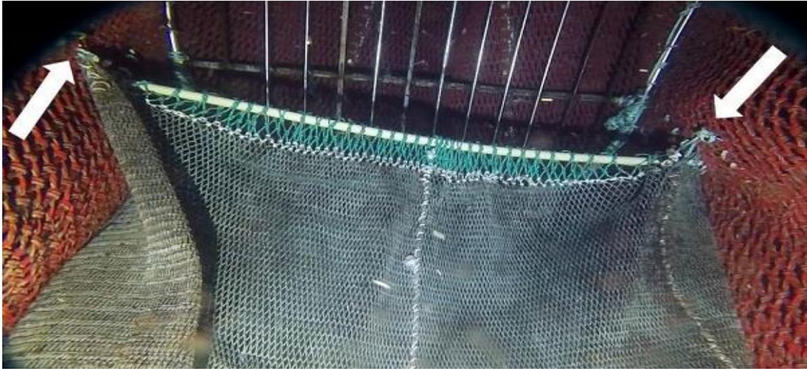
**Fig.7.** Compliant SED-B. The arrows indicate the attachment of the small mesh panel to the sides of the net. The internal escape hole is neither blocked by ropes nor mesh. Note the PVC tube in the border of the panel.
