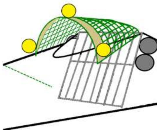
**Fig.4.** Diagram of hood SED. The hood is made by 90mm mesh; conveyor belt material is attached to its edge to work as a kite. Three 30mm buoys maintained the hood in position and the escape hatch open. The green dotted line represents the internal mesh panel.
