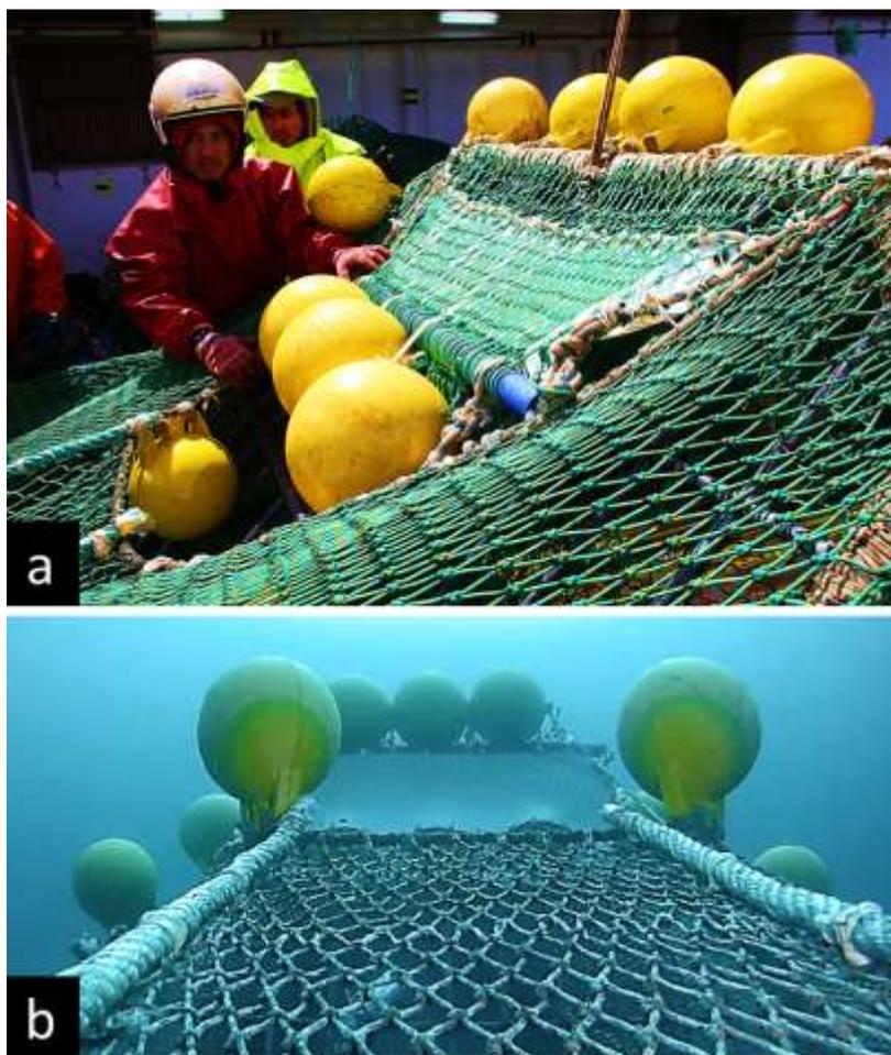
**Fig.7.** Visor SED. On deck view (a) and after deployment (b), with visor's buoys entangled with SED's top flotation.
