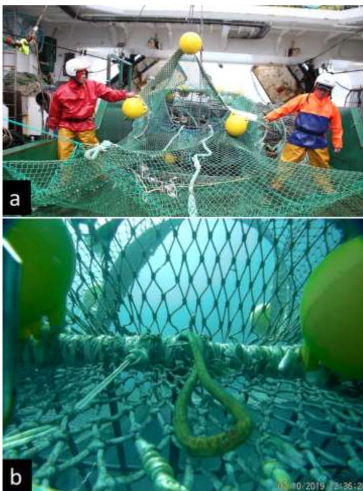
**Fig.5.** Hood SED. Open up on deck (a) and hood's rear view after being deployed (b).
