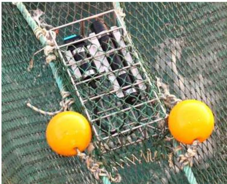
**Fig.13.** Protective netting on top of the external housing.
