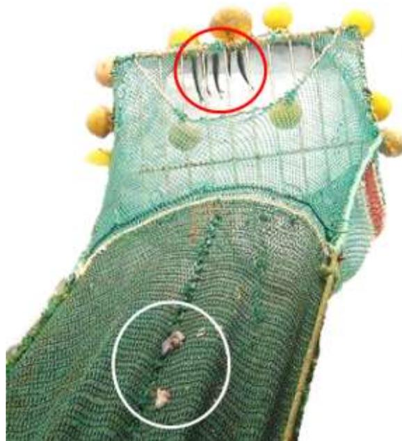
**Fig.2.** Fish loss through SED in a finfish vessel. The position of the enmeshed fish indicates an upward current flow through the hatch. Note the short SED's next extension; it is unknown whether this SED had either a mesh panel or a high-speed funnel to canalise the water flow through the grid towards the cod-end.
