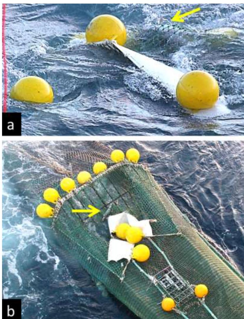
Fig.16. Hood behaviour in the surface during hauling. During manoeuvring the hood mostly remains open (a). While being close to the vessel and outside the water, the hood collapses (b). The yellow arrows indicate HAK retained in the hood.
