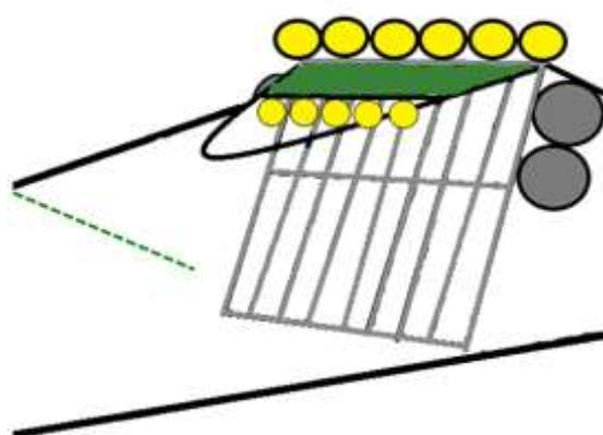
**Fig.6.** Diagram of visor SED. The visor is made of conveyor belt material and covered by netting. The green dotted line represents the internal mesh panel.
