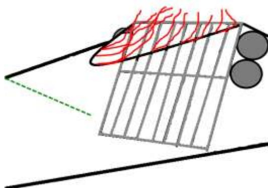
**Fig.8.** Diagram of streamer SED. The streamers are made of red semi-flexible polyurethane 10 mm tubing. The green dotted line represents the internal mesh panel.
