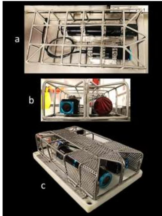
**Fig.11.** Trawl housings. Protective structure mostly used inside the SED (a, b). Note the cellophane filter in torch (b). Protective footage kit housing used on top of the net (c). Note the higher coverage of the cylinders and the Teflon base.
