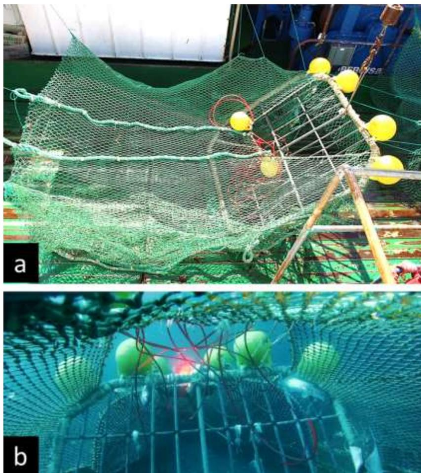
Fig.9. Streamer model. On deck view (a) and after deployment (b).
