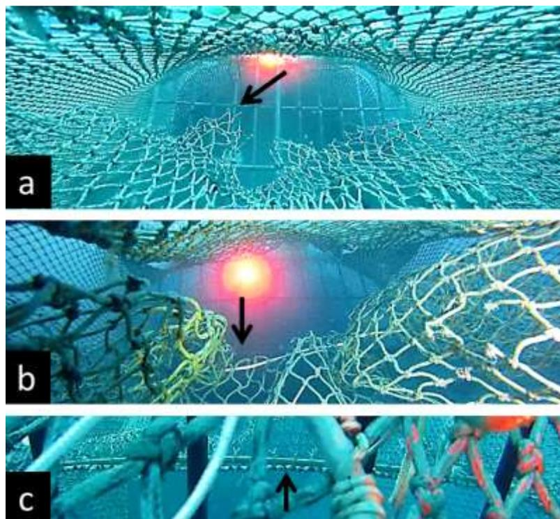
**Fig.3.** Internal mesh panel. Original loose configuration (a), early modified version with a string (b), final configuration with a rope inside a PVC tube that connected the mesh panel to the sides of the net extension (c).
